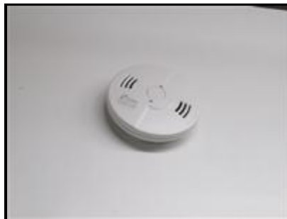
A. Picture 1 CO Monitor / Mechanical Room
